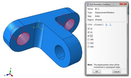
Now we define a load in the form of a surface traction – this is a force per unit area in a defined direction.
