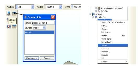
Whilst the solution is running we can monitor its progress. Right click the job and select 'Monitor'.
