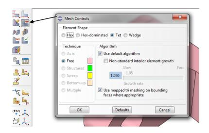
Click the 'Mesh Part' option to apply the mesh options to the part. The viewport will automatically update to display the meshed part.
