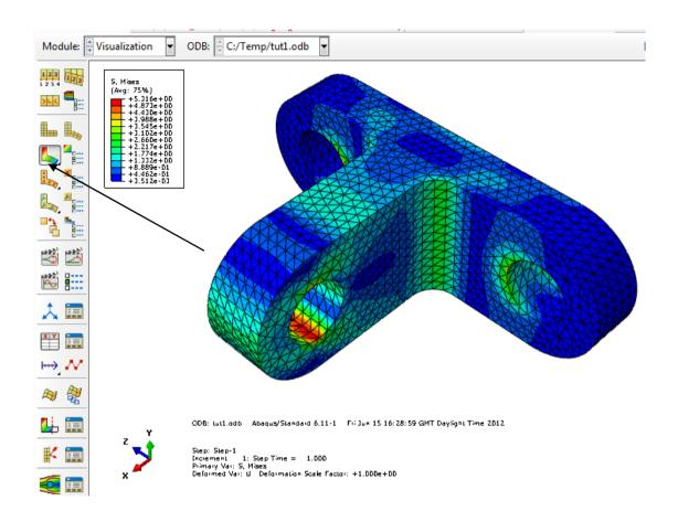
Take time to explore the contour plot post-processing options, try creating a displacement plot for the model.
