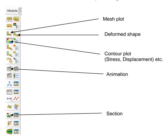
Now we wish to create a stress plot of the model. By selecting the 'Results' -> 'Field Output' from the menu bar we can select different post processing quantities to plot on the model. We want a Von Mises Stress plot.
