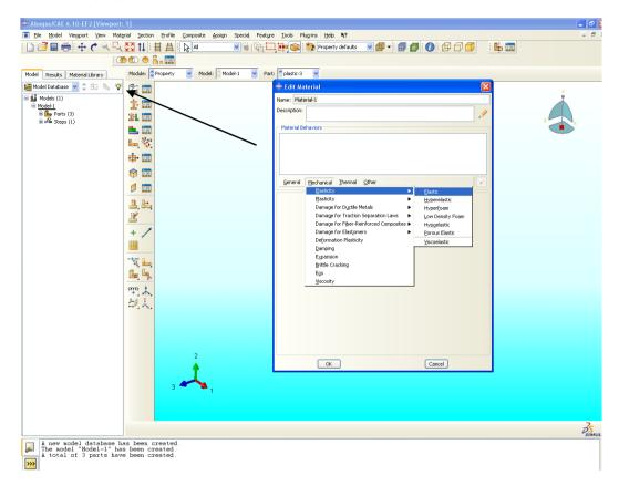
We define a modulus of 70e3 (Newton and mm units – remember to be consistent). Also define a Poisson's ratio of 0.28.
