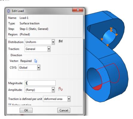
With a surface traction we need to specify a direction in which the force should act.
