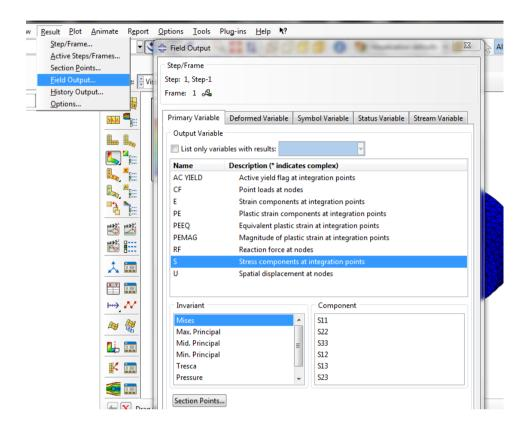
Once we have selected what we require the contour plot to show we can apply it to the model by selecting the 'Plot Contours' option.
