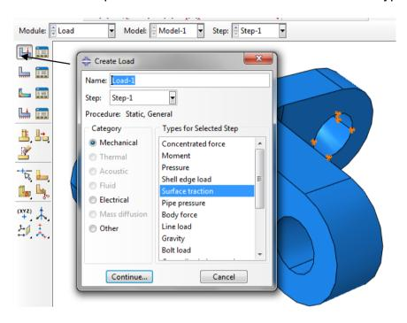
Using the same method as before select the face highlighted in the image below and then enter a magnitude of 1 and set the traction type to general in the Edit Load window.
