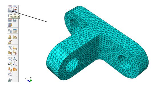
If necessary the mesh can be locally refined using local mesh seeds. Before a local mesh seed can be applied we need to delete the current mesh.
