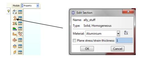
This section then needs to be applied to the geometry. This is how we tell the software which parts are made of what.
