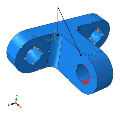
Now we have created a 1N surface traction in the X-axis direction.
