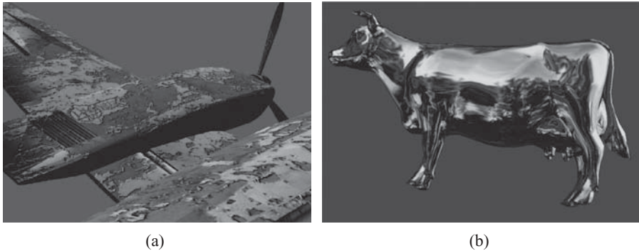
Figure 7.25 Other texture mapping methods include (a) bump mapping and (b) environment mapping (courtesy of OpenSceneGraph).
