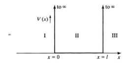
Potential energy function V(x) for the particle in a one-dimensional box
