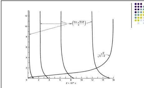
Graphical solution of the equation  $tan(2\pi L\sqrt{2}mE/h) = \sqrt{E}/\sqrt{U} - E$ . Here L = 2.50 nm, m = 9.11 × 10–31 kg, U = 1 eV = 16.02 × 10–20 J. Intersections occur at E = 0.828×10–20 J, 3.30×10–20 J, 7.36×10–20 J and 12.8×10–20 J.
